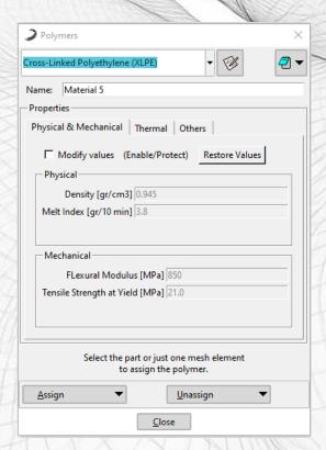
Once the polymer and its appropriate property values have been chosen, the polymer must be assigned to the geometry.
