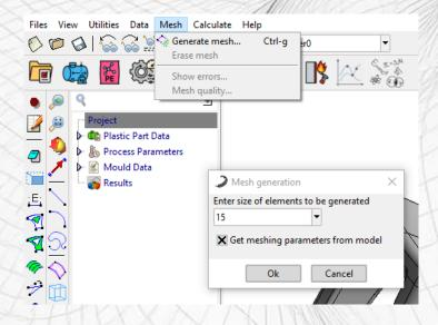
When generating the finite element mesh, it is important to carefully choose the element size. A mesh that is too coarse can compromise the quality of the results, while an excessively fine mesh can generate an unnecessary number of elements, increasing computational costs without providing significant improvements.
