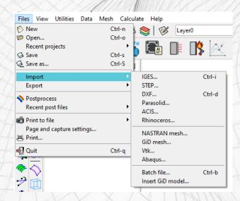
The geometry to be imported must be a closed 3D CAD part, solid or shell. In the case of a shell, there must be no thickness.
